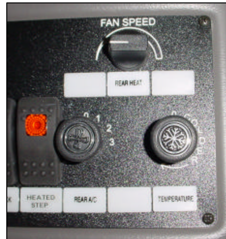
Figure 6: Switch Panel Optional A/C & Heat Controls for Passenger Compartment Comfort
