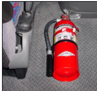
Figure 63B: Fire Extinguisher Installed Next to Driver's Seat
