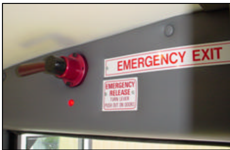
Figure 14: Front Entrance Door Emergency Release Handle
