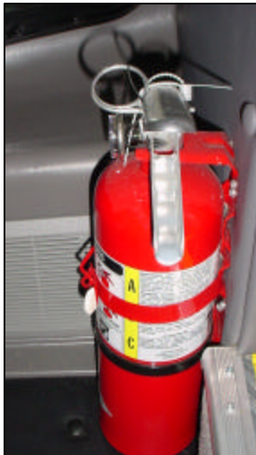
Figure 63A: Fire Extinguisher Installed Next to Entrance Door
