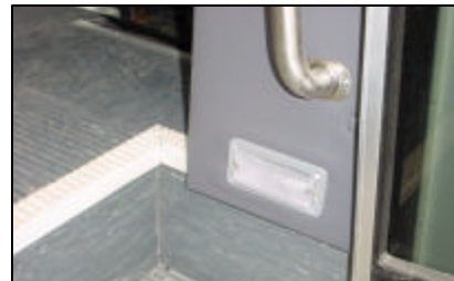
Figures 8B: Step-well Lights on Side of the Steps
