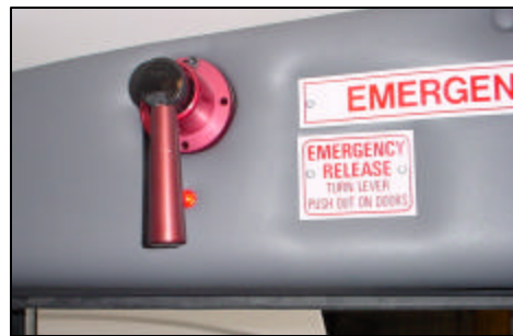
Figure 15: Front Door Release Handle in Door Open Position
